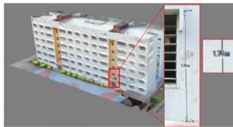
Figure 4. Drone Application; a) Slope Mapping, b) Building's Crack Measurement
